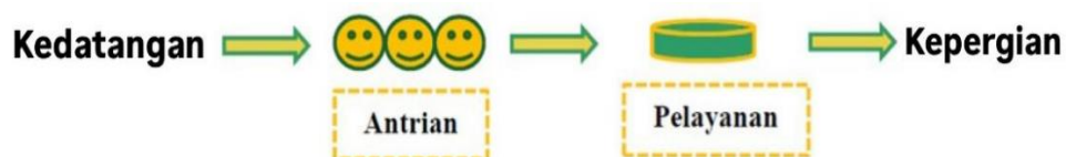
Gambar 2.6: Model single channel-single phase (Aseha dkk, 2023)
