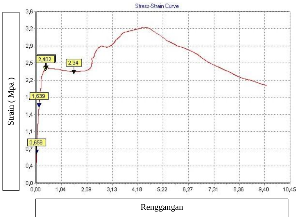
Gambar 4.11 Grafik Stress Strain Beton ASPSTIII
