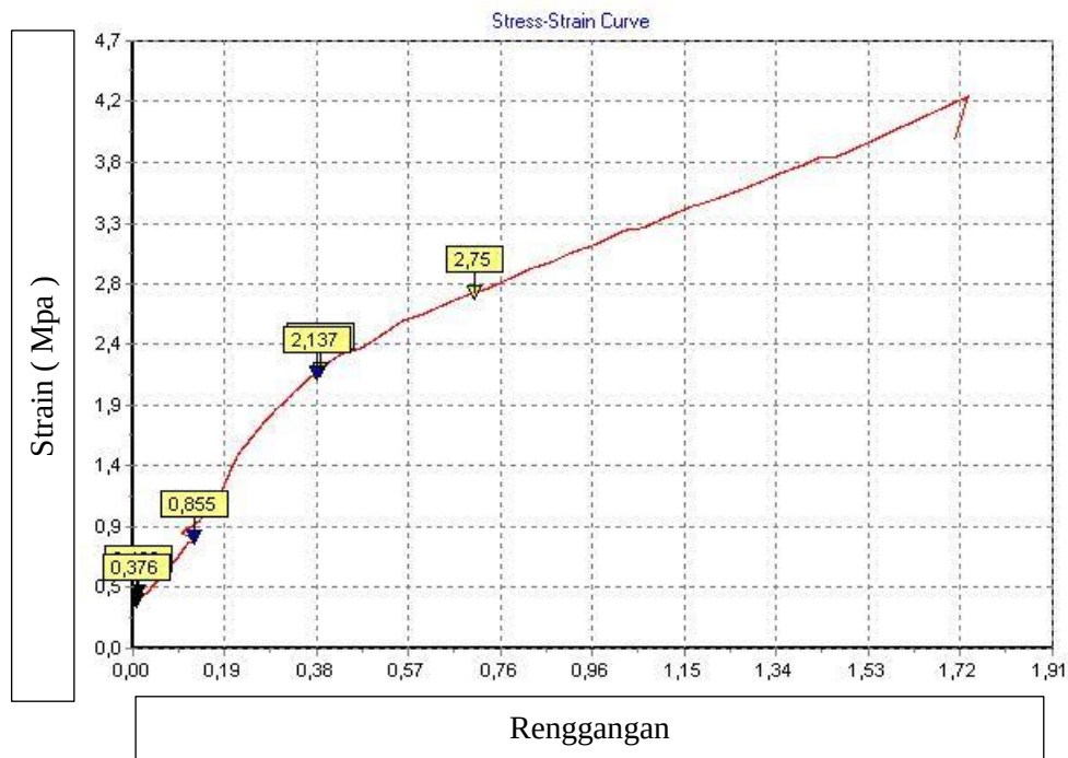
Gambar 4.9 Grafik Stress Strain Beton Serat tebu
