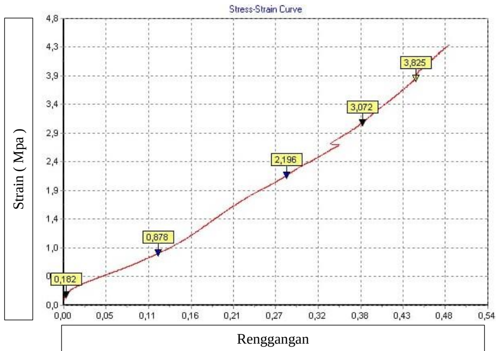
Gambar 4.10 Grafik Stress Strain Beton ASPST I
