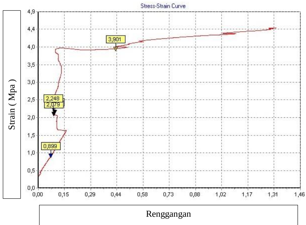
Gambar 4.11 Grafik Stress Strain Beton ASPST II
