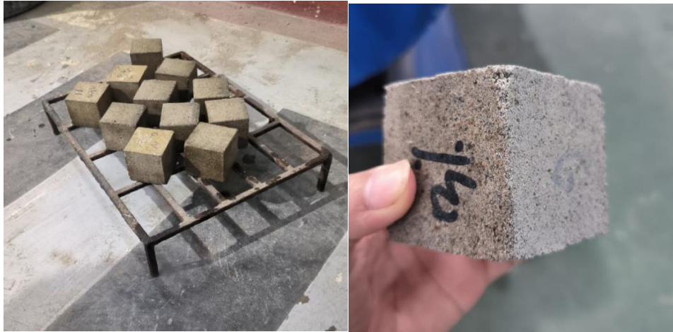
Gambar 4.13: Hasil Pengujian Efflorescence
