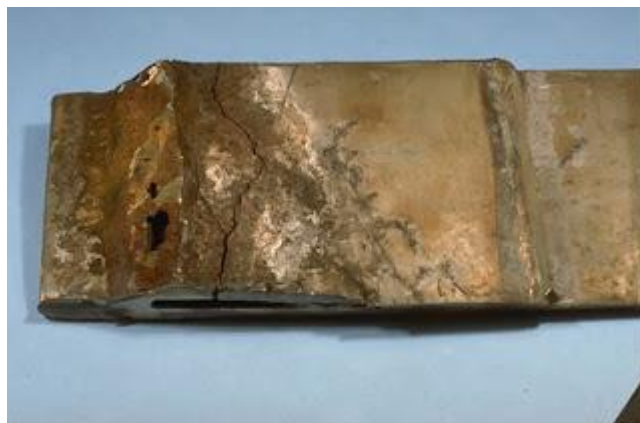
Gambar 2.8 Stress Corrosion Cracking (SCC) (Utomo, 2012)
