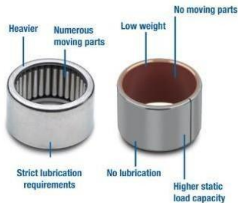
Gambar 2. 16 Plain Bearing ( https://www.indiamart.com/proddetail/needle-rollerbearing )
