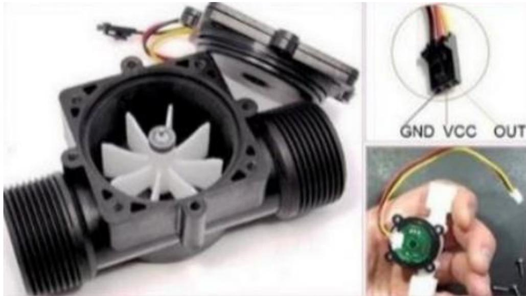
Gambar 2. 10 Sensor Flowmeter
