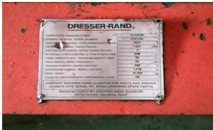
Gambar 3. 1 Nameplat Gas Engine
