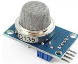
Gambar 2. 6 Modul Sensor MQ135
