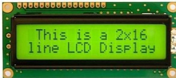
**Gambar 2.4 LCD16X2**
