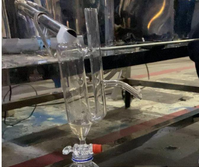
Gambar 3. 10 *Essential Oil Hydrosol Separator*
