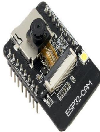
Gambar 2. 2. ESP32-Cam
