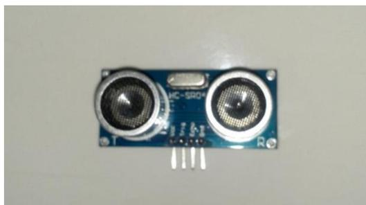
Gambar 2. 9. Sensor Ultrasonik HC-SR04
