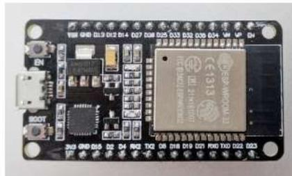
Gambar 2.4 Mikrokontroler ESP32(Makrup, Amalia Herlina, and Fuad Hasan 2022)
