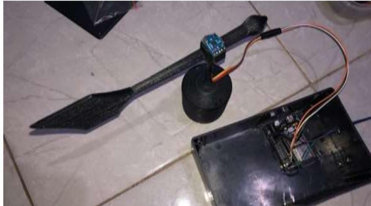
Gambar 4.16 Menghubungkan pin sensor ke board esp32
