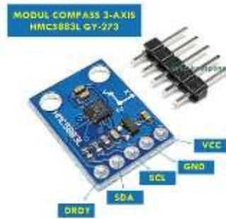
Gambar 3.4 Sensor HMC5883L
