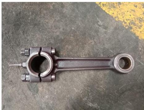
Gambar 2. 10 Batang Engkol (*Connecting rod*) Mesin *Diesel*
