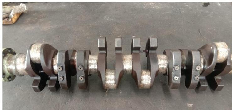
Gambar 2. 11 Poros Engkol (*Crank Shaft*) Mesin *Diesel*
