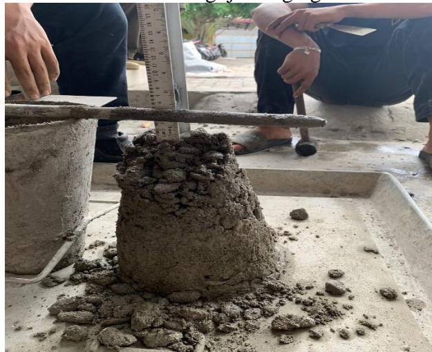
Gambar L- 4: Perhitungan Nilai Slump
