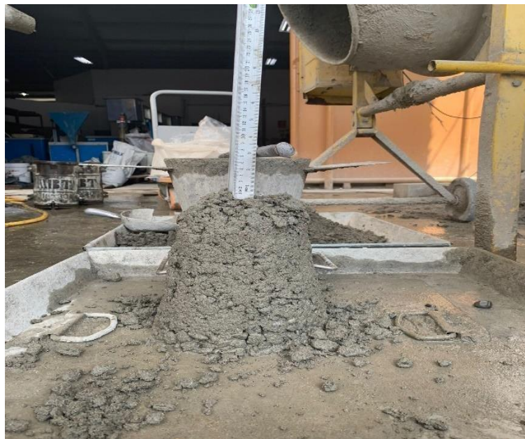
Lampiran 6: Pengujian Slump
