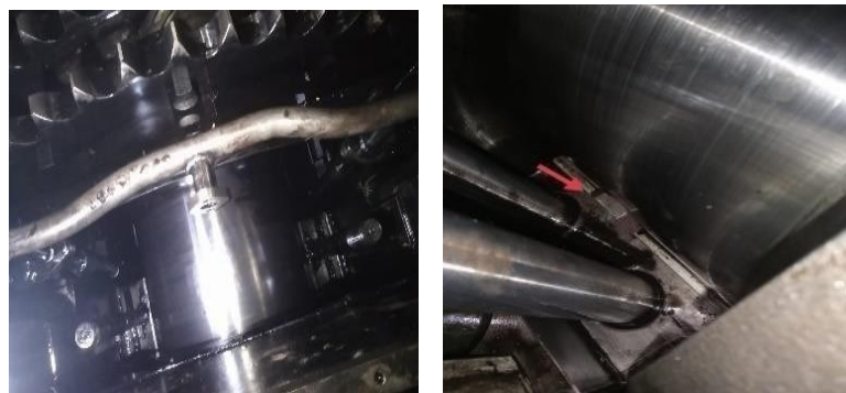
Gambar 4.14 Proses pembongkaran lower Main bearing (PT. Waruna Shipyard Indonesia)
