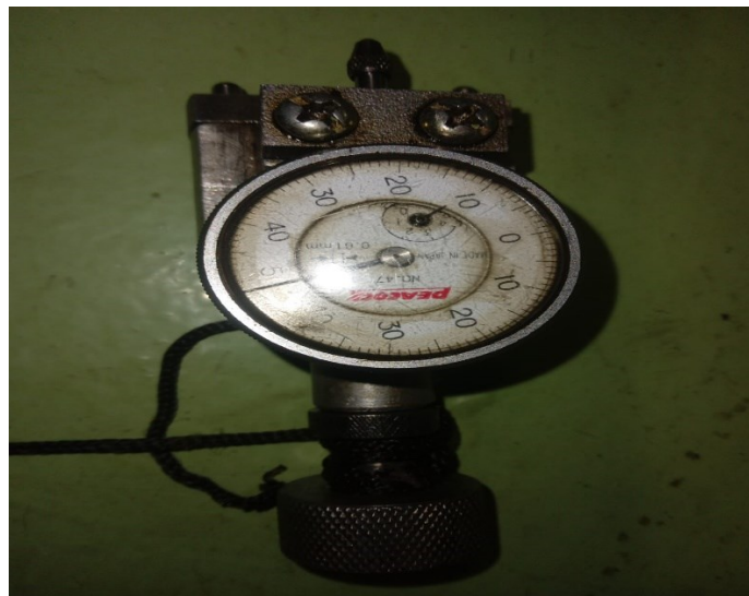
Gambar 3.8 Dial Deflection (PT. Waruna Shipyard Indonesia)
