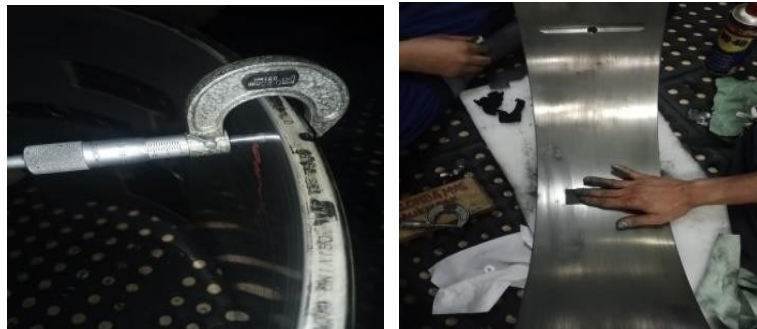
Gambar 4.13 Proses cleaning bearing dan pengukuran (PT. Waruna Shipyard Indonesia)
