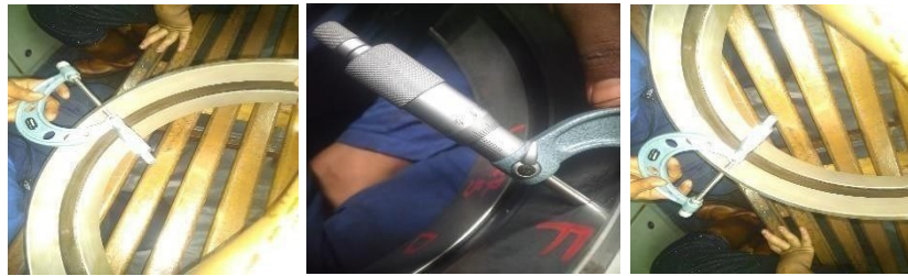
Gambar 4.15 Pengukuran thickness metal main bearing (PT. Waruna Shipyard Indonesia)
