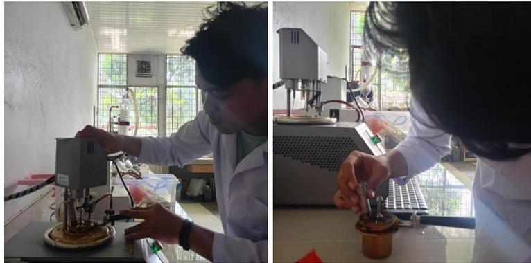
Gambar 3.11 Proses Pengujian *Flash Point*
