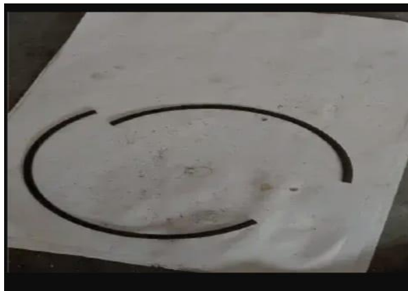
Gambar 4.4.1 Patah Ring Piston
