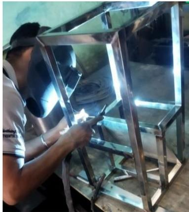
Gambar 4.5 Proses Pengelasan Alas Tungku
