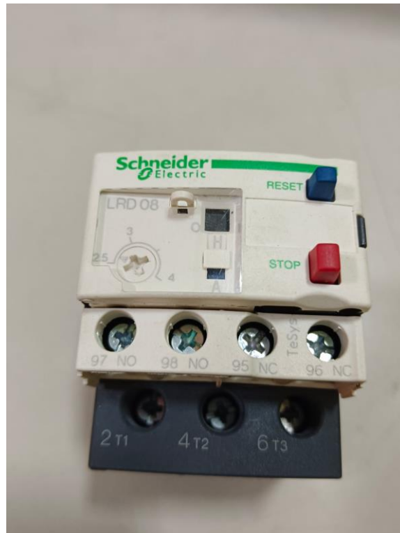
Gambar 2. 12 Thermal Overload Relay (TOR)
