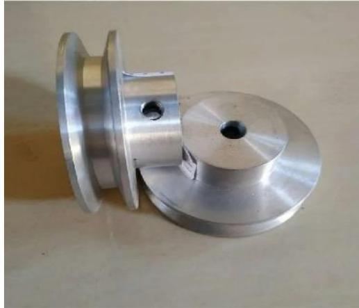
Gambar 2. 4 Pulley Alumunium
