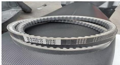
Gambar 3. 14 Transmisi sabuk (*V belt*)
