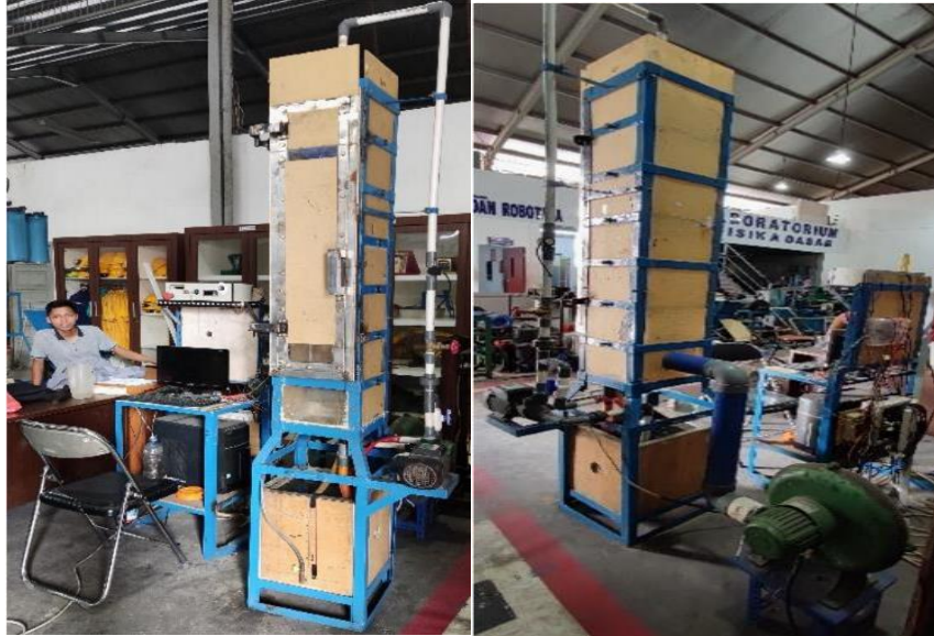
Gambar 3. 1 Prototipe Cooling Tower
