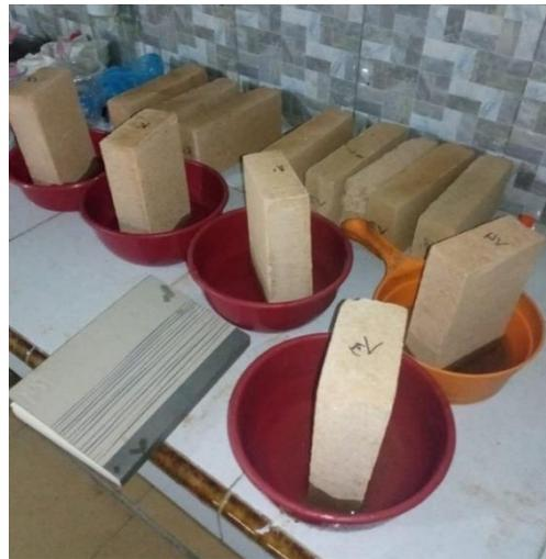
Gambar 4.5: Proses pengujian kadar garam
