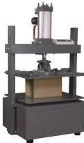
Gambar 3.12 Compression test
