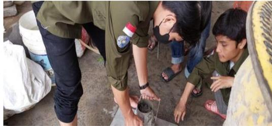
Gambar 3.27 : *slump flow*
