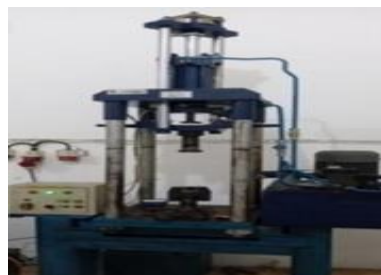
Gambar 3.1 Mesin Uji Tekan ( Universal Testing Machine )
