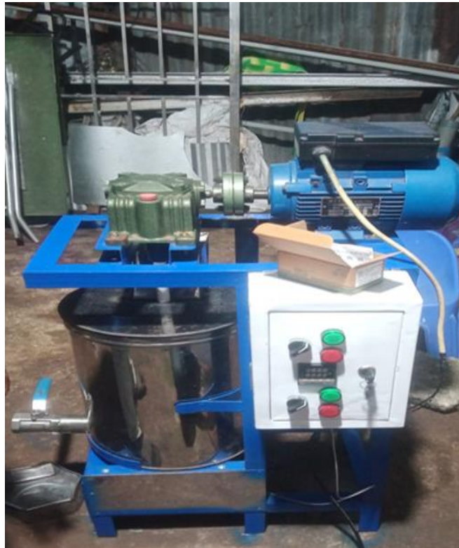
Gambar 3.8 Mesin Paving Block Berbahan Dasar Plastik
