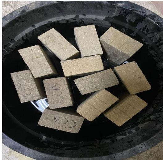
Gambar 4.25: Proses benda uji dilakukan pengujian kadar garam.
