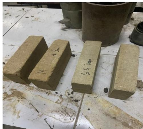
Gambar 4.26: Benda uji hasil pengujian kadar garam.
