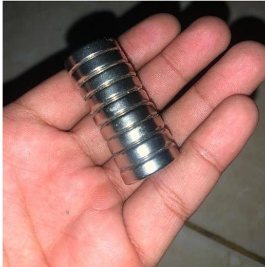
Gambar 3.7 Magnet *Neodymium grade N52* ukuran 20mm x 5mm
