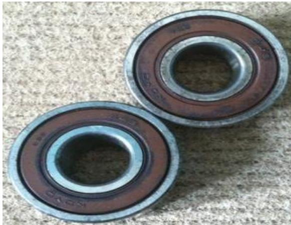
Gambar 3.10 *Bearing* / Laker diameter 2cm
