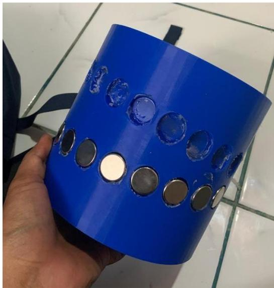
Gambar 3.8 Desain Drum / Rotor
