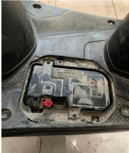
Gambar 3.21 Socket *DLC* ( data link conector)
