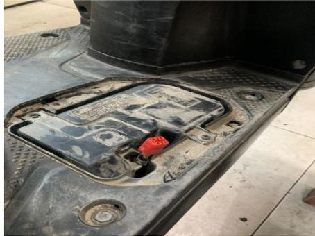
Gambar 4.13 Socket DLC ( data link conector)
