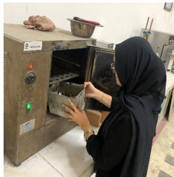
Gambar 3.3: Pengujian kadar air
