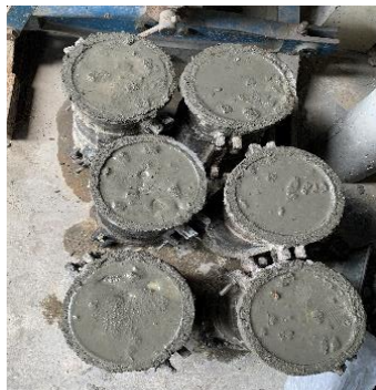
Gambar 3.13: Benda uji beton silinder
