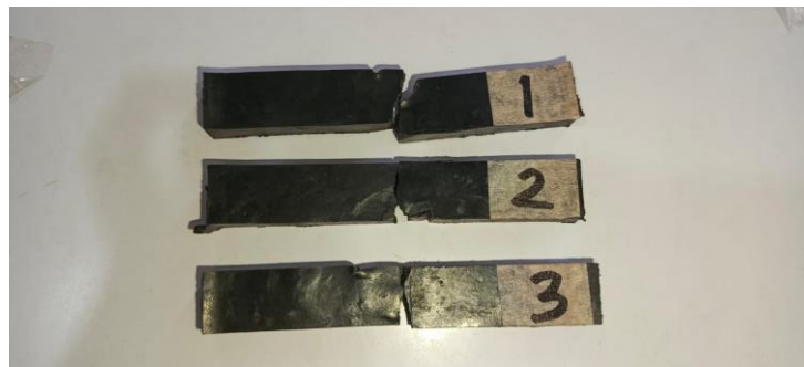
Gambar 4. 21 uji impact 70% hdpe :25% karet alam dan 5% abu boiler
