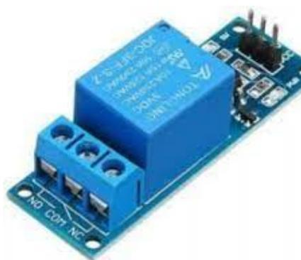
**Gambar 2.13** *Relay* 1 Channel
