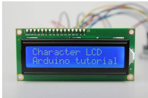
**Gambar 2.11** LCD 16x2
