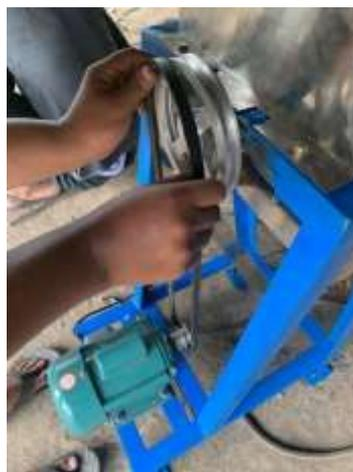
Gambar 4.16 Proses Pemasangan V'Belt Ke Pulli
