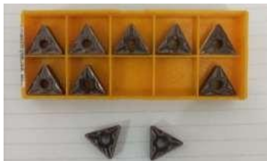
Gambar 3.2 Triangle Insert Turning Type T
