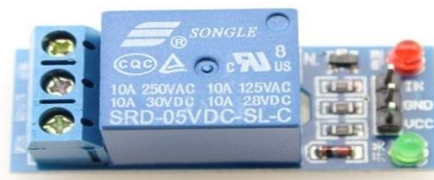
Gambar 2. 11 Modul Relay 5 VDC (Rachmatullah et al., 2018).
