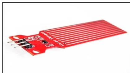
Gambar 2. 8 Sensor ketinggian air (Hidayat & Nasution., 2014)
