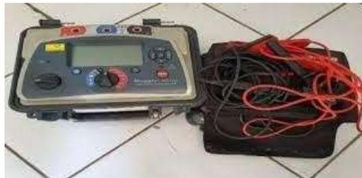
Gambar 3.1 Insulation Tester merk Megger, Tipe MIT1025
