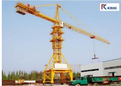
Gambar 2.8: Rail mounted crane (Krhicranes, 2022)
