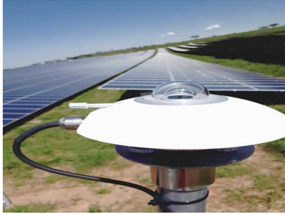
Gambar 2.8 Pyranometer
