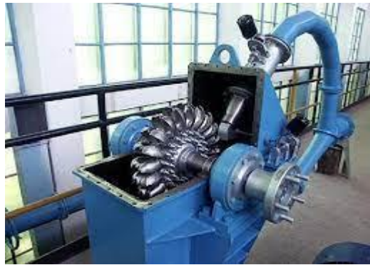
Gambar 2. 9 Turbin Peleton (Irawan, 2014)
