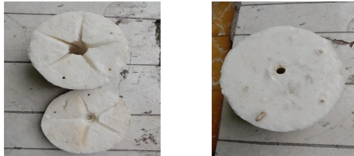
Gambar 4.1 Hasil Molding Sudu-Sudu Turbin Kaplan
