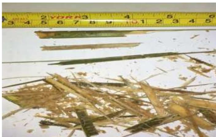
Gambar 4.16 Ukuran cacahan  $\geq 50$  mm
