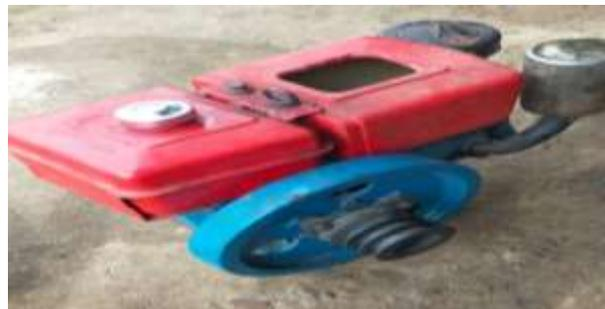
Gambar 3.8 Motor Diesel
