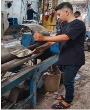
Gambar 4.33 Proses Pengerolan Plat *Stainless Steel*
