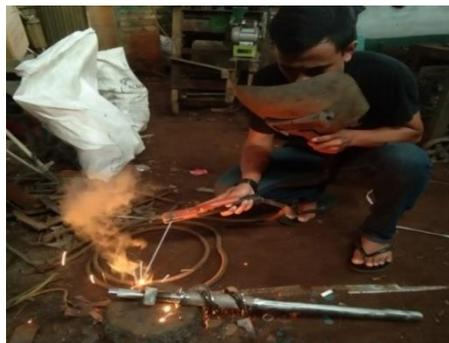
Gambar 4.32 Proses pengelasan ulir as *screw*
