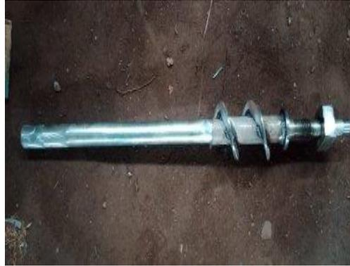
Gambar 4.33 Hasil pengelasan ulir screw dan as
