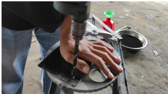
Gambar 3.5 Melubangi plat alumunium
