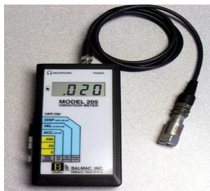
Gambar 2.23 Balmac Vibration Meter Model 200M
