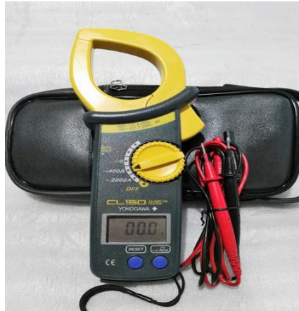
Gambar 2.24 Clamp On Tester YOKOGAWA CL-150
