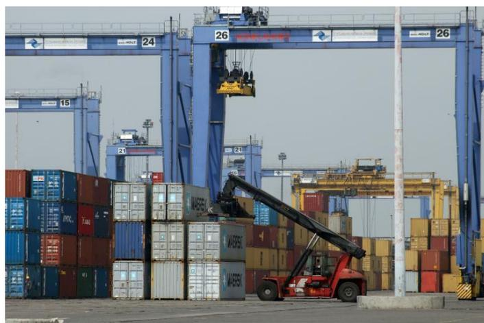
Gambar L 3. *Rubber Tired Gantry Crane*
