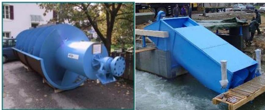
Gambar 2.2 Turbin Screw (a) Tipe Steel Strough dan (b) Tipe Closed Compact Installation (Saefudin dkk., 2017)
