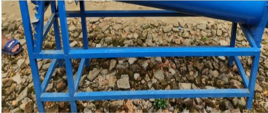
Gambar 2.4 Rangka Turbin Archimedes Screw
