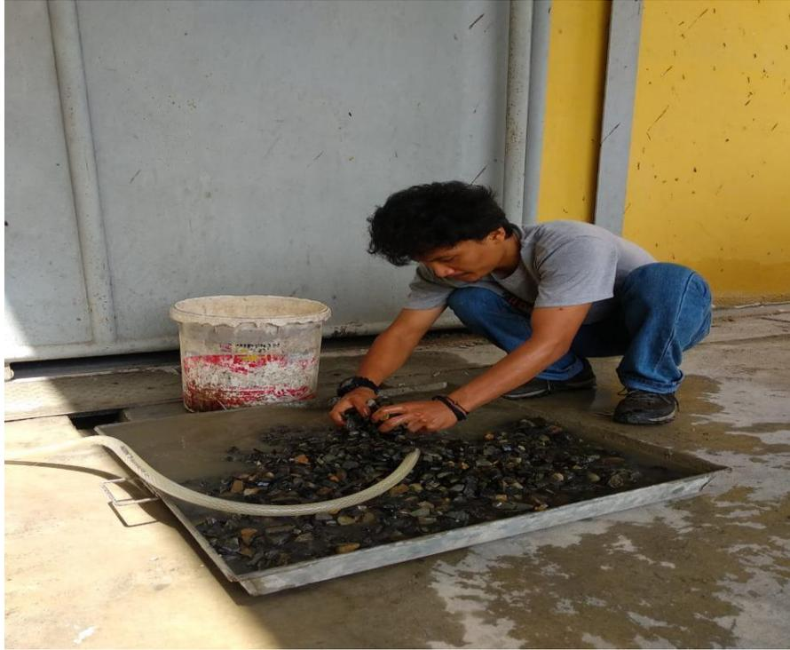
Gambar Lampiran 1. Pencucian agregat
