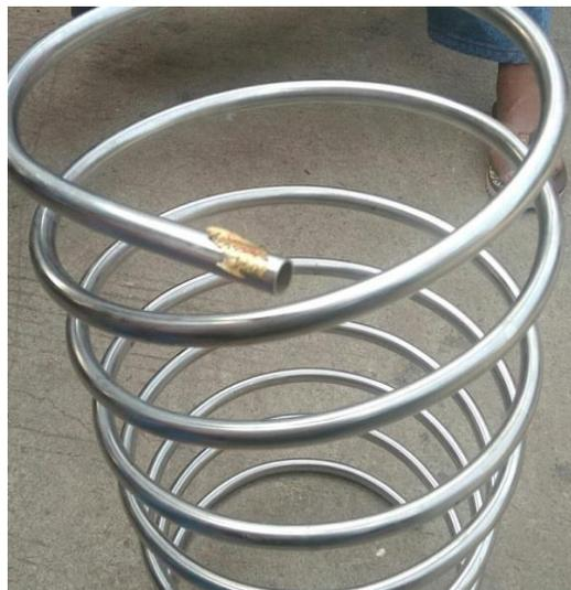
Gambar 2.8 Pipa Spiral (*Heat exchanger*)
